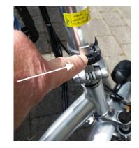
PEDALS can be folded by putting finger through centre ovel hole in pedal and compressing in direction of the arrow.
