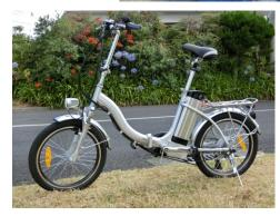
Remember to switch key off after use. Tyre Pressure Front 45 lbs rear 50lbs
